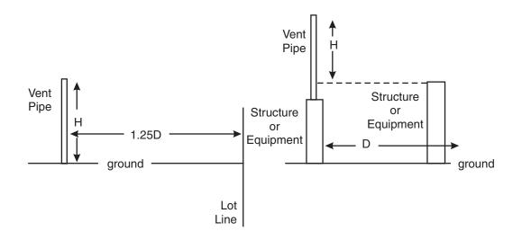
H = Minimum height in feet of vent pipe above the ground or above any structure or equipment within distance (D) where personnel might be present. D = Distance in feet to adjacent structure or equipment where personnel might be present.
